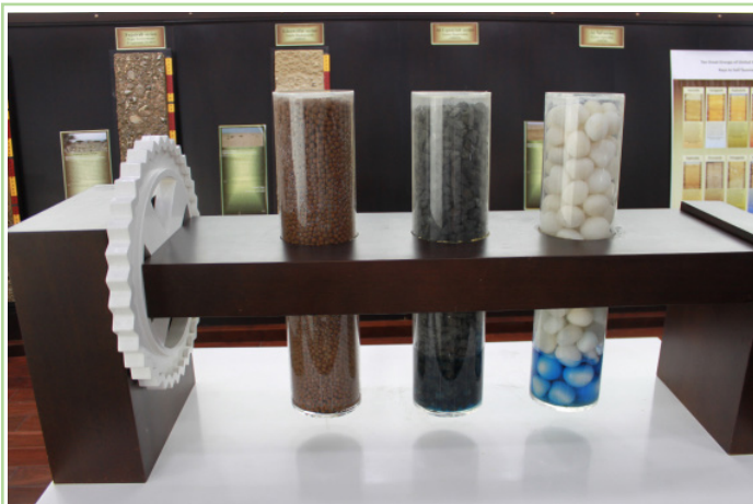
The Water Infiltration Simulation Unit demonstrates how sizes of soil particles (sand, silt, clay) in soil influence infiltration rate.
