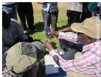
Measuring soil salinity, part of the practical field training at ICBA
