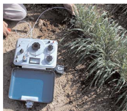
In-situ salinity measurement by salinity bridge.
